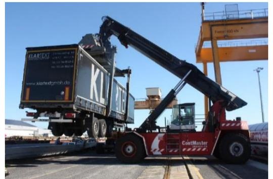
The future rail motorway terminal will use an intermodal technology (loading & unloading standard trailers - and craneable ones - in dedicated wagons) allowing a modal shift of trailers to ease the transition from road to rail and increasing maritime volumes.
